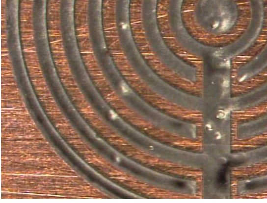
Fig. 1. Microstructure with 0.25\text{mm}^2 of area, included in a silicon wafer. In this case the device is a capacitor that can be applied for different situations and goals.
