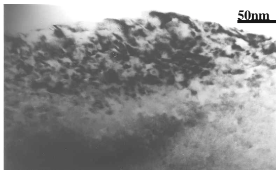
Fig. 9 Cross-sectional transmission electron micrograph with (001) and (111) planar defects.
