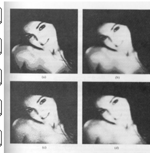
(a) image digitized with only 16 gray levels (exhibits false contours); (b) result of smoothing (a) with a lowpass filter of order 1; (c) noisy image; (d) results of applying Butterworth lowpass filtering to the noisy image.
