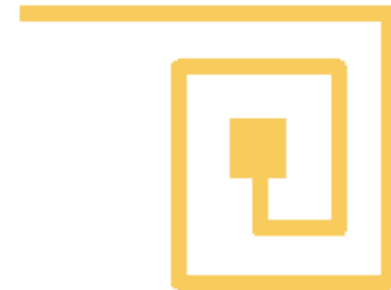
Example for designing an inductor on LTCC
