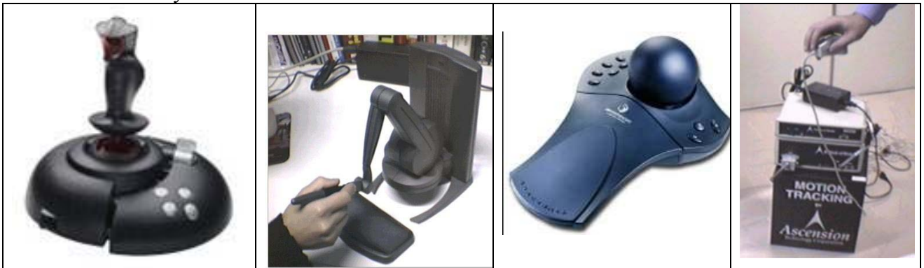
Some Interactive tools : Joystick, Haptic, Spaceball and a Motion Tracker 3D.
